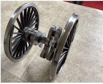
The Photo below shows one of the Bogie Axles. If you look closely, you can see the joint between the casting and the tyre on the circumference.
