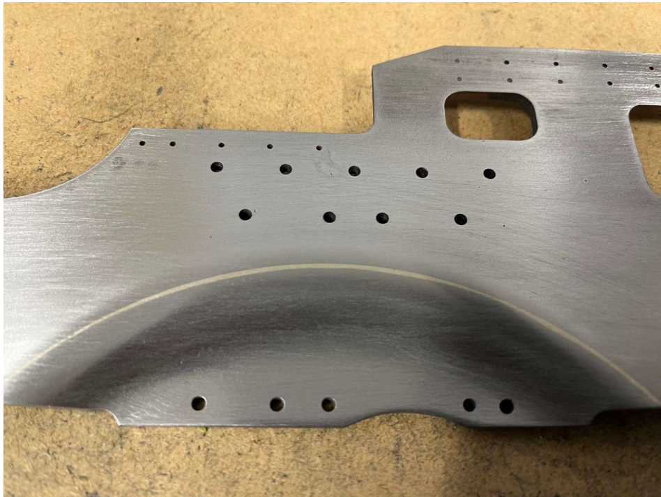
Photo 3 - Dished section in place
