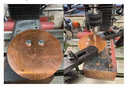
Using a centre finding point the centre punch for the main flue was located, the whole assembly then clamped down for drilling.
