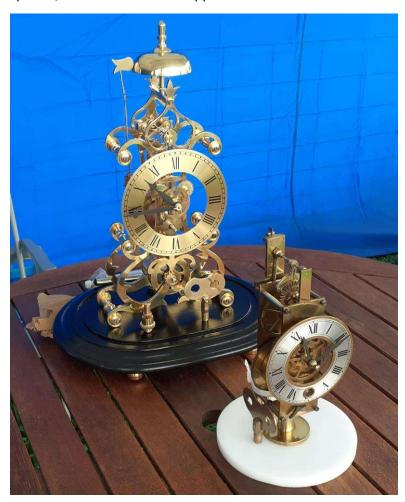
For most of us the idea of cutting the rather ornate chassis/ mainframe would have been a major contract. Not for Keith as he had other ideas. One top tip from Keith was to plan ahead before starting the cutting operation. With the price of brass sheet these days you could be wasting a lot of scrap material, whereas smaller components could be manufactured from offcuts. Another interesting operation was creating a thread on a cone shape. (Excuse my spelling, this cone shape was called a fusee).
