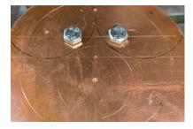
All the holes were marked out, on one plate only and then I drilled two holes that will be used for the 1/4" stays that go the length of the boiler, these holes were used to fix the end plates together for drilling.
