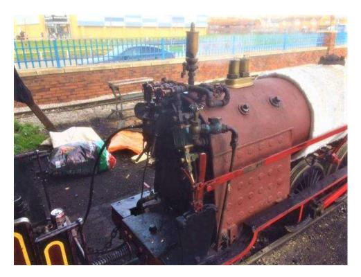
The steam pipework on the backhead looked as if it was made from steel electrical conduit. If it was, it's lasted very well over the years. I was asking how many times they would have to add coal to the fire on one circuit of the track and was surprised to be told the only time they add coal to the fire is at the station before starting the journey.
