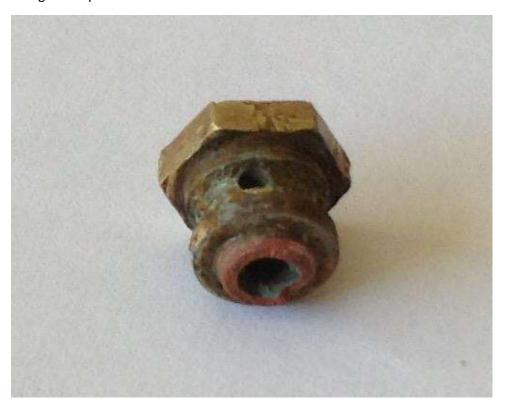
This boiler will need pickling in something similar to white vinegar or kettle de scaler, then thoroughly flushing out before any movement under steam. The holes you can see in the banjo are 1/16"dia. A very bad design, I'm hoping I'll have sufficient clearance from the wheels to put an elbow in place of this design.
