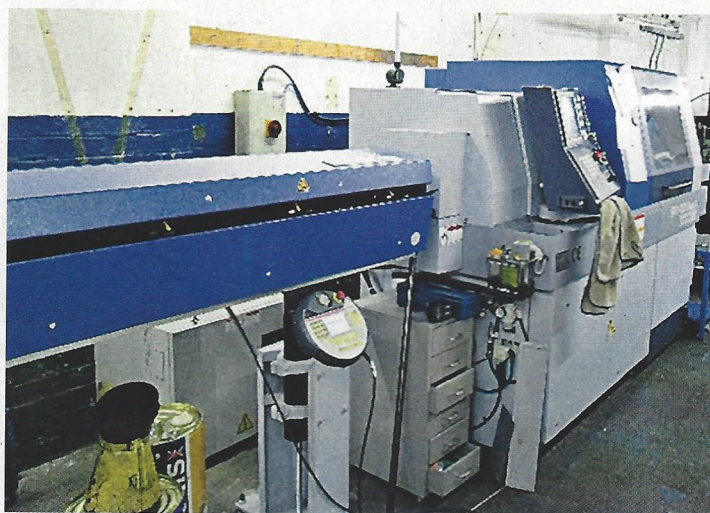
Star. A major investment in the future of model engineering added to the well equipped workshop. A 7-axis sliding head lathe, capable of accurately producing the most intricate parts.
