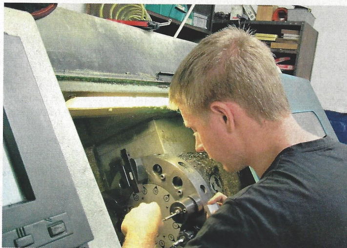
Matt Tornado. Matthew Andrews, an apprentice trained at Polly, confidently setting the tools in a Tornado CNC lathe.
