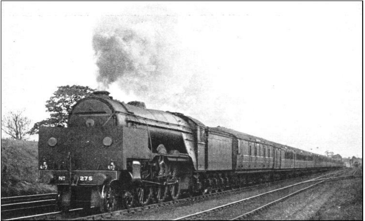
THE INDICATING SHELTER - Attached to the front of a "Pacific" locomotive undergoing tests. Members of the engineering staff ride in this compartment for the purpose of taking indicator diagrams of the expansion of the steam in the cylinders and collecting various smoke-box data.
