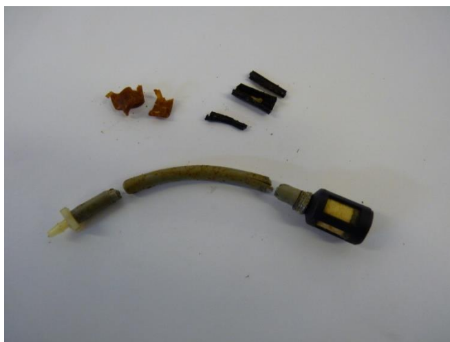
Parts found in the trimmer petrol tank.
