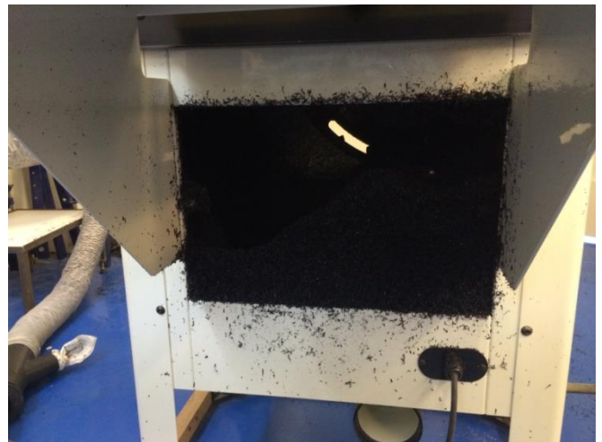
Photo h The blocked up saw
