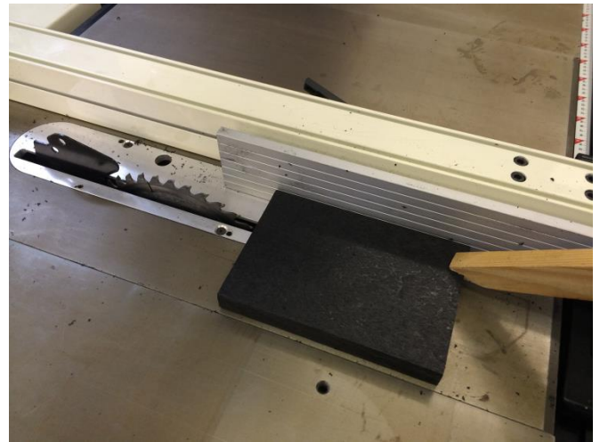
Photo b Cutting the blocks into sleepers
