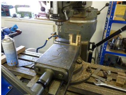
How not to hold a hornblock
