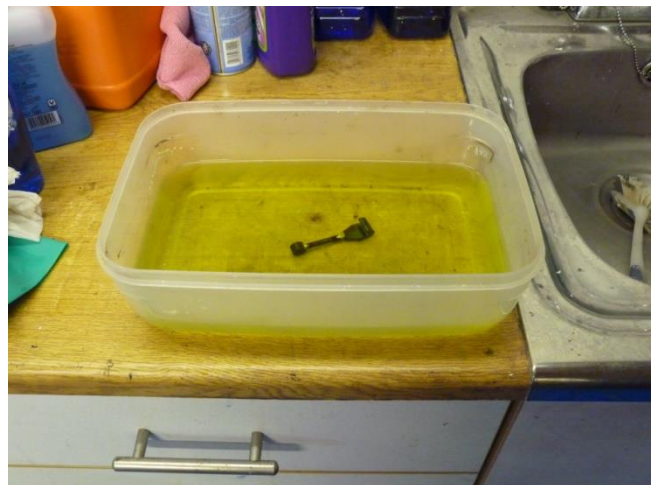
Hanger soaking in Hydrate 80
