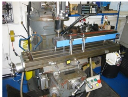
The column mounted on the mill
