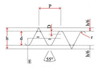
P = Pitch = 1/Number of threads per inch (tpi)  $h = Angular Depth = 0.960491 \times P$   $D = Depth of Rounding = 0.073917 \times P$   $h/6 = Shortening = 0.160083 \times P$   $d = Actual Depth = 0.640327 \times P$   $r = Radius at the Crest & Root = 0.137329 \times P$   $C = Core diameter = Major Diameter - 1.280654 \times P$ Effective or Pitch Diameter = Major Diameter - .640327 \times P
