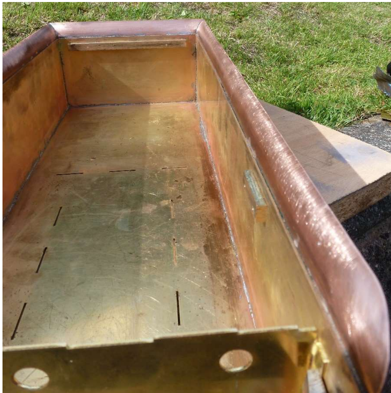
Sections mitred, rounded and soldered into position
